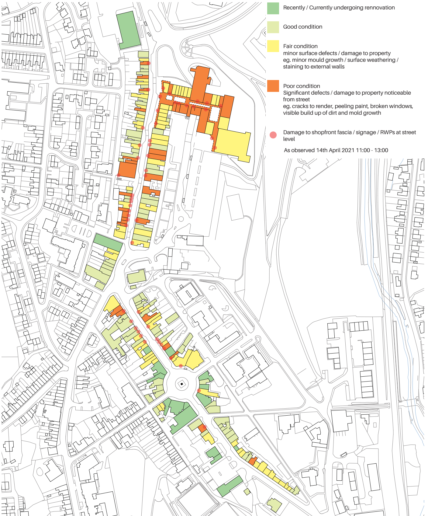
FIG. 6 BUILDING CONDITION SURVEY
